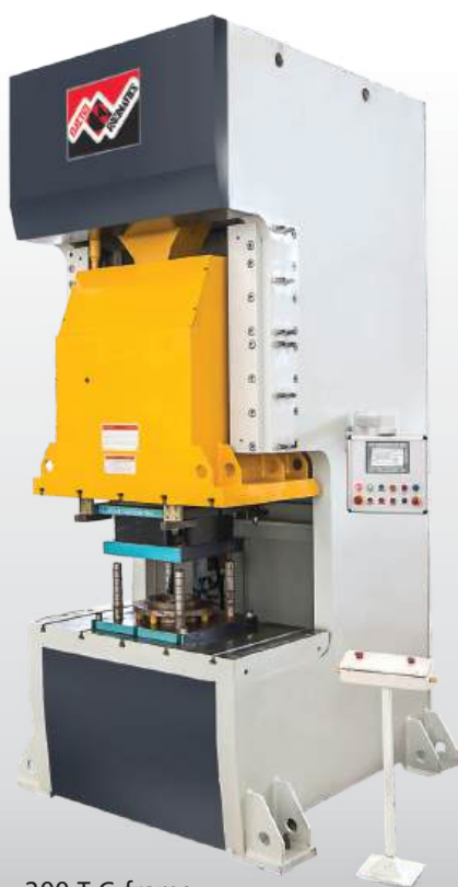
200 T C-frame servo mechanical press
