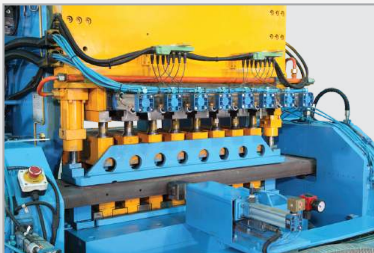
CNC chassis web and flange punching machine with automatic in-feed and out-feed conveyors
