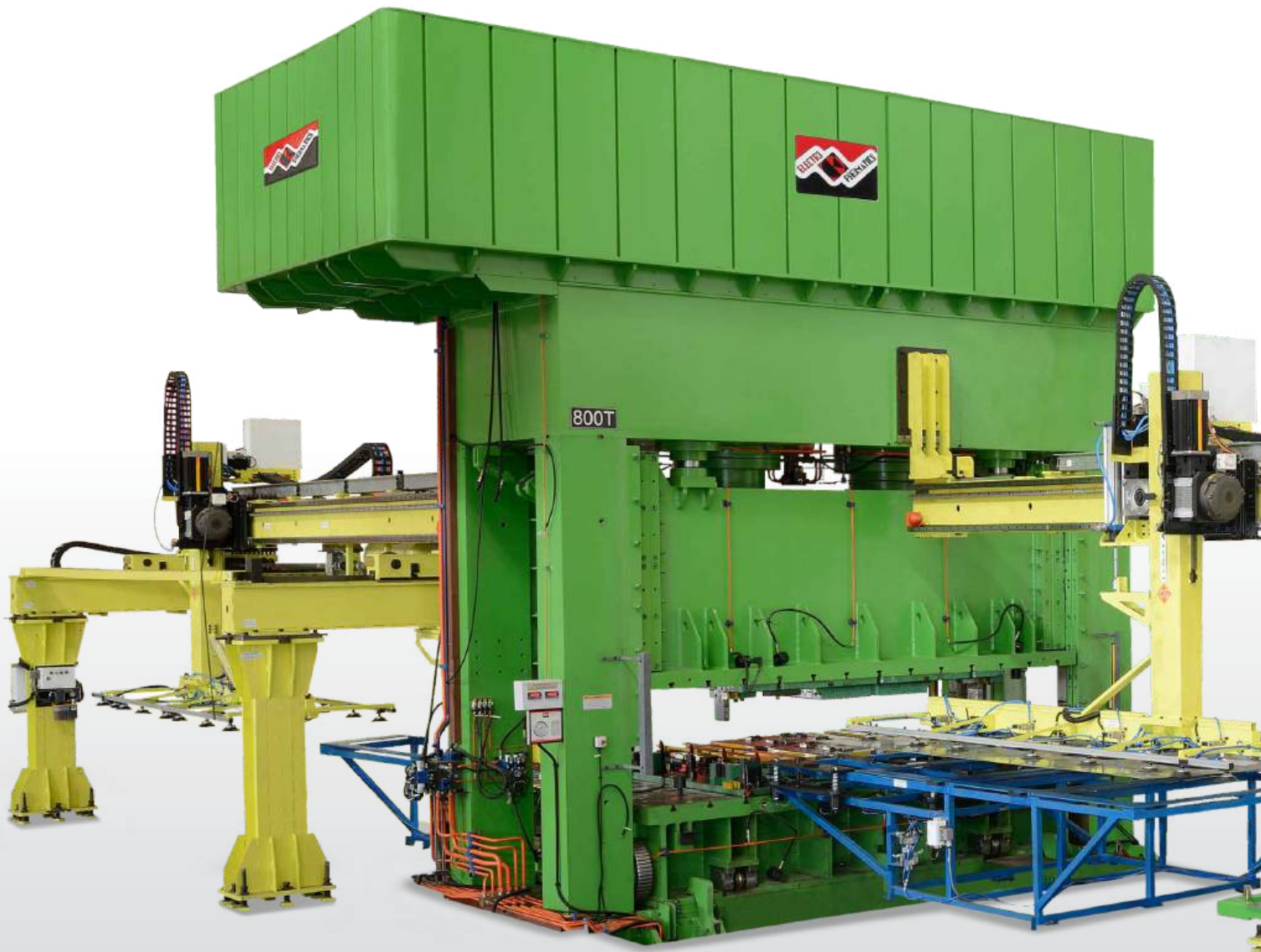
Fully automated 800 T hydraulic press with sheet loader and unloader for trimming and forming of railway coach body side panels
