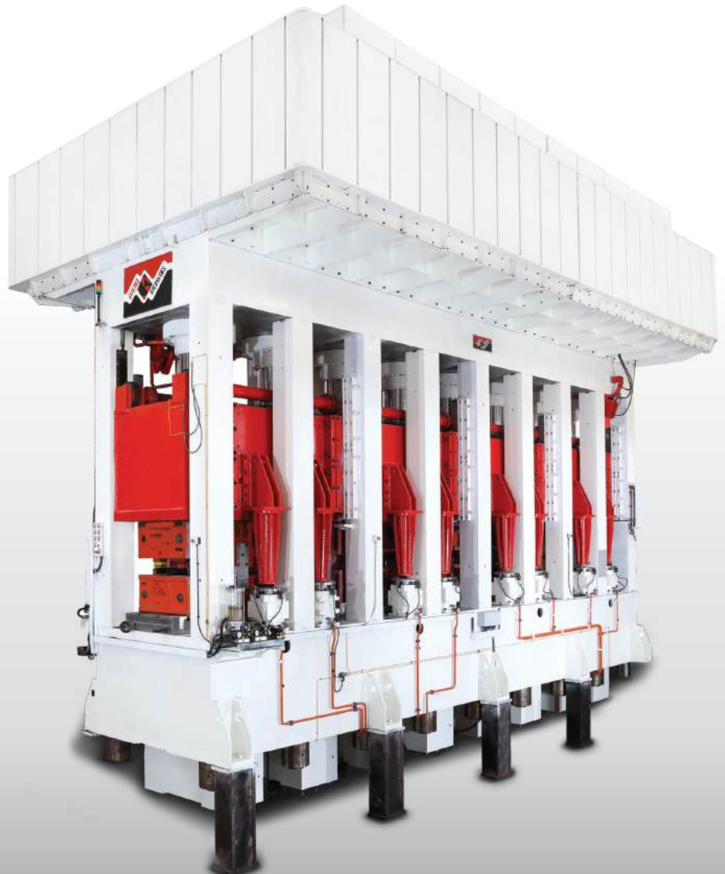
4500 T hydraulic press with two independent slides and die cushions for forming and punching chassis long member
