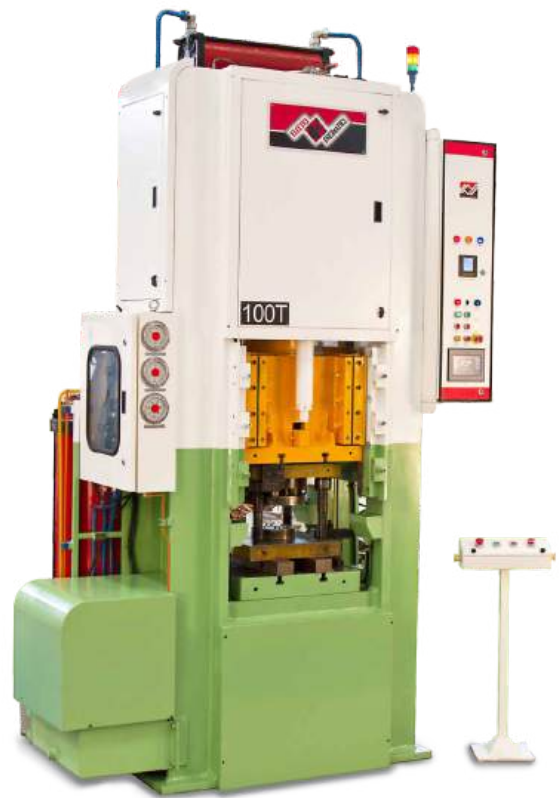
100 T straight sided servo mechanical press
